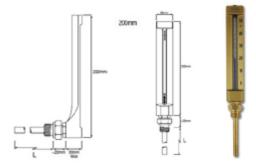
The user needs to determine the 'L' length, by checking how much the stem needs to be inserted into the pipe or engine in order to measure the temperature. The 'L' length measures the distance from the top of the thread to the tip of the stem.
