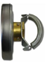
When installing the thermometer, it is vital that a good connection is made between the sensor on the back of the thermometer and the pipe. If the sensor is not sitting flush against the pipe an incorrect reading may be obtained. If the pipework is too small, the sensor will not make full contact with the pipe. Clip on pipe thermometers that are 63mm in diameter are generally used on pipework between 20mm and 50mm.
