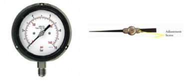
Other pressure gauges may have an adjustment screw on the needle itself. The cover and window need to be removed and a screwdriver used to turn the needle into position. You must hold the needle still while turning the screw and it must be done carefully as the needle is connected the spring and is very sensitive. The gauge could become permanently damaged if care is not taken when performing this adjustment.
