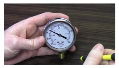
Some pressure gauges have a screw on the dial face, either behind the needle or by the scale of the gauge. To access this, remove the cover and the window. Then either turn the screw clockwise or anticlockwise to return the needle to zero.
