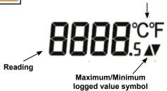
Three different functions are available on the display - most recent logged temperature, maximum logged temperature and minimum logged temperature. The push button is used to cycle through the functions. In addition, logging and alarm status are shown using two high intensity LEDs.
