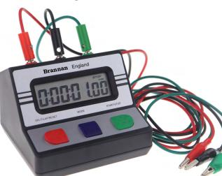
The Brannan bench top timers are easy to use and are particularly suited for use in schools. They have colour coded buttons and a clear LCD display, designed to offer accurate measurement over a long period of time.
