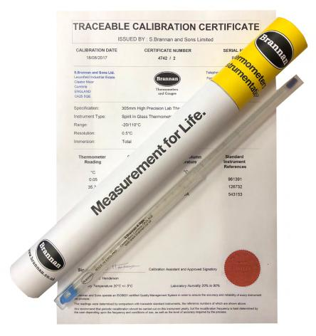
The **THERM***cert*<sup>TM</sup> range of liquid-in-glass thermometers are calibrated at two or three separate points across their working range. These thermometers are supplied complete with a traceable calibration certificate and are presented in a sturdy cardboard cylinder for storage.
