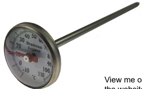
\* The thermometers will operate at shorter immersions, however the stated accuracy cannot be maintained.
