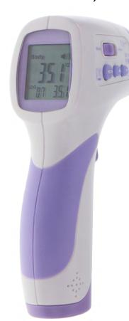
Non-contact and hygienic infrared thermometer specially designed to take the body temperature of a person regardless of room temperature. The thermometer has a fast response time allowing a greater number of measurements to be taken in a short time.
