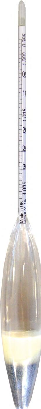
The American Society for Testing and Materials (ASTM) Specification E 100 describes hydrometers using the API (American Petroleum Institute) scale and others in degrees Specific Gravity.
